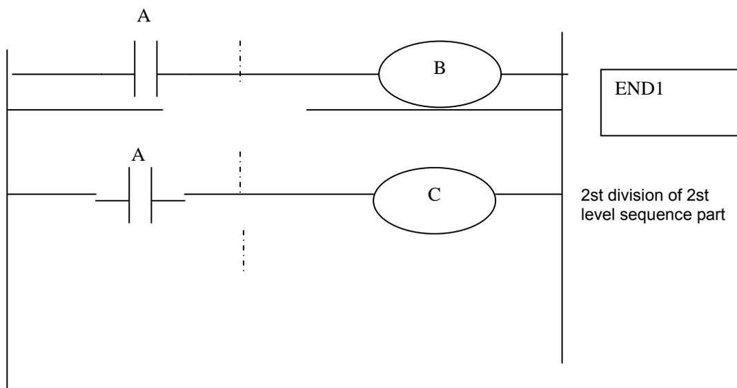
When the processing is 1st 4ms, A=1, and B=1 after 1st sequence part is executed. At the same time, 2nd sequence part is started to execute A=1 is stored to the 2nd sequence part and the 1st division of 2nd sequence part is executed.
