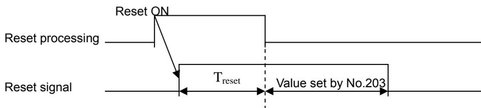
When the CNC is reset in automatic operation, the automatic operation is stopped and movement axis is decelerated and stopped. When the CNC is reset during the execution of the M, S, T function, signal MF, SF or TF is set to 0 within 16ms.
