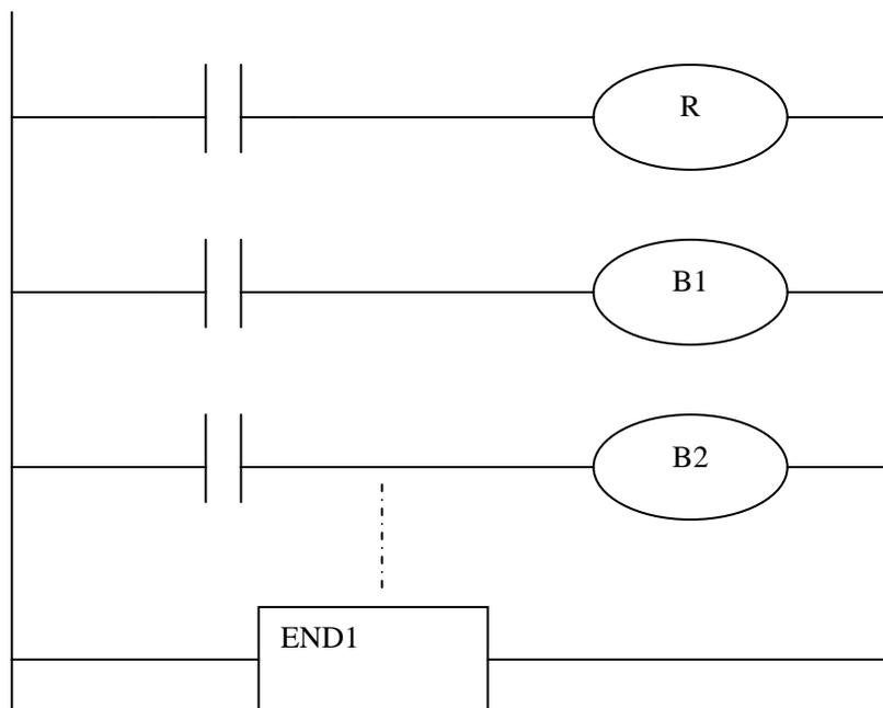
B1 and B2 are not 1 simultaneously after the signal A is processed synchronously by the medium relay.
