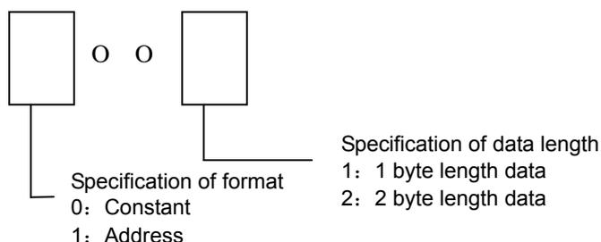
S1, S2: content of comparison source 1 and comparison source 2. It can be constant and also be address number.
