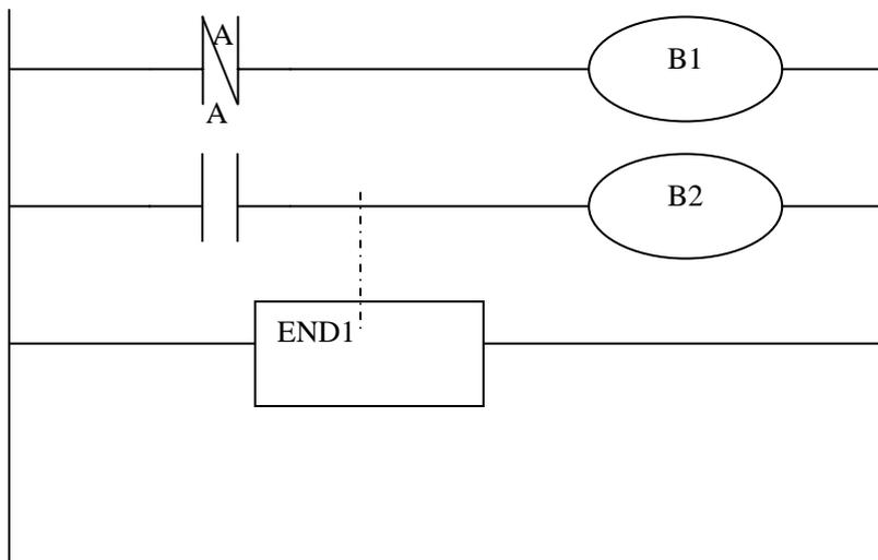
When A=0, and B1=1, A becomes 1, at this time, the next line of ladder is executed, B2=1. B1 and B2 are also 1
