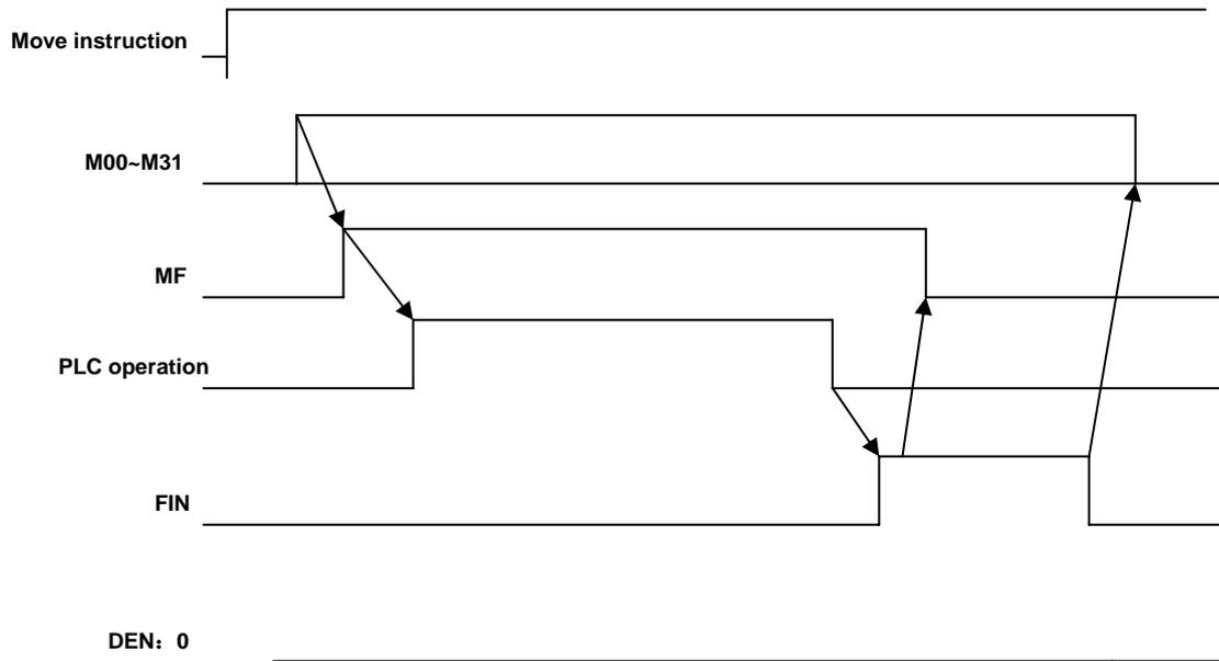
Move instruction and a miscellaneous function during the same block. Execution of a miscellaneous function after move instruction completion:
