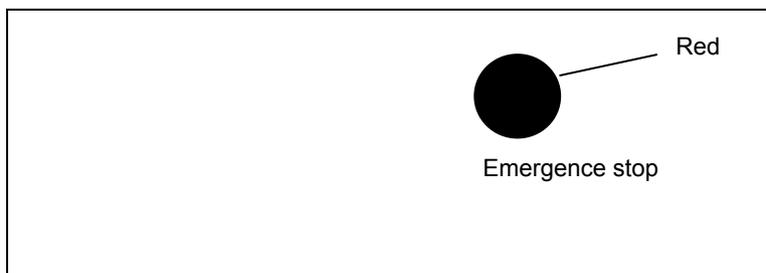
The button is locked when it is pressed, Although it varies with the machine too builder, the button can usually be unlocked by twisting it.
