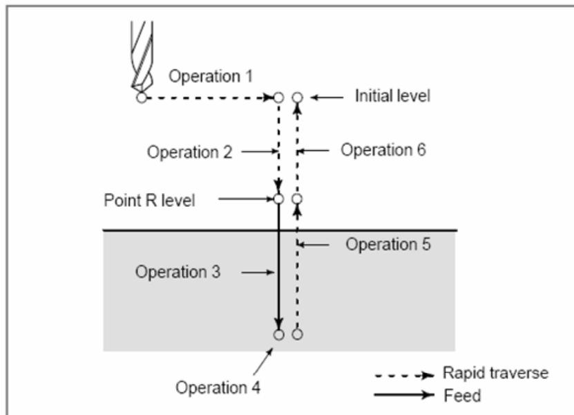
The following canned cycles require spindle control:
