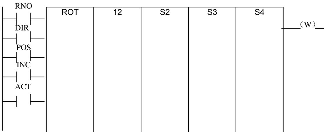
Perform the short path rotation, and calculate the position number of previous one position of goal position.
