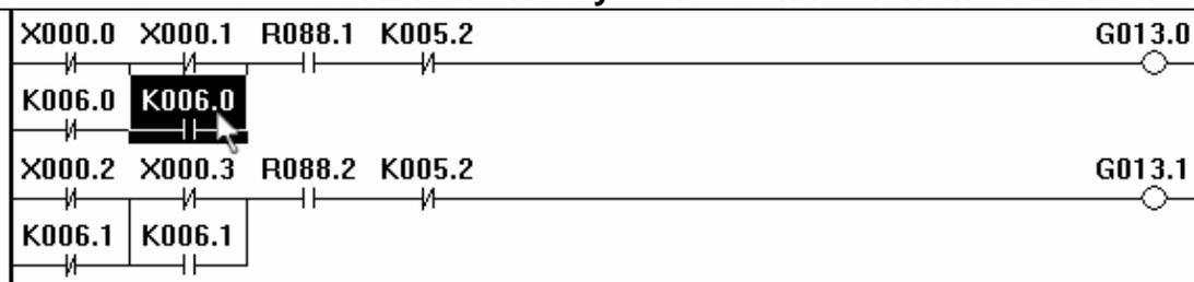
When the block is selected, the user should press the left key of mouse in its initial position to drag the mouse to the end of the row, and the surroundings of the selected area is appeared by a rectangle with many dotted line before releasing the key.
