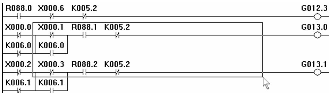
After the mouse is released, the whole ladder becomes black, i.e., the ladder in the range is selected, and the user can execute the next operation, such as clip, delete, copy and so on.
